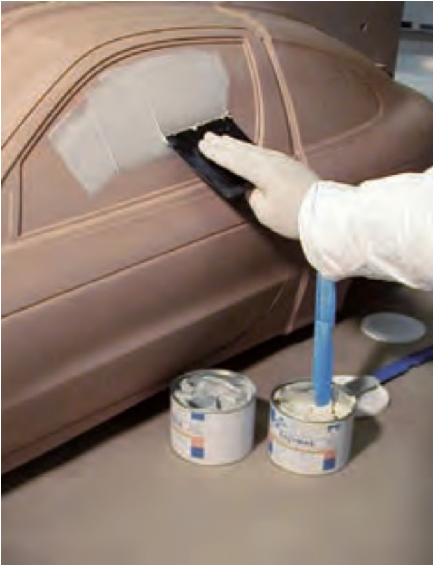
Easymax perfect match repair putty to medium density boards having the same PUR chemistry with quick setting and odour-less
