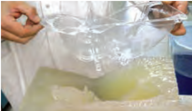
Elastic mould produced by addition curing silicone Essil 291 for optical parts
