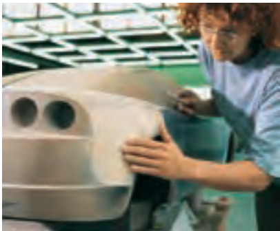
Models milled out of SikaBlock® PROLAB 65 fulfil highest demands of surface quality
