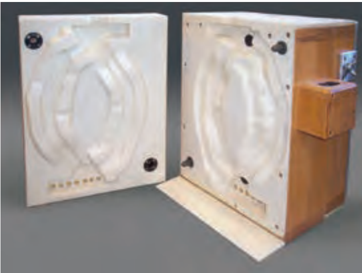
Core box made of SikaBiresin® UR322 NT
