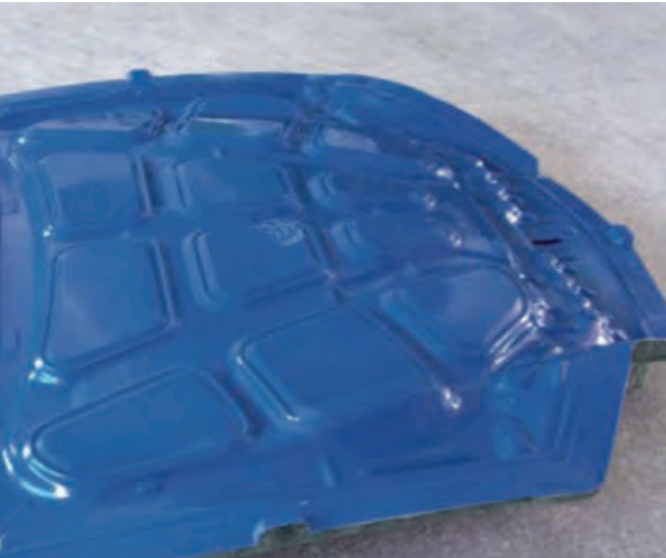
Tool for making reinforcements of bonnets made of SikaBiresin® GC080
