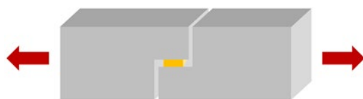
Figure 12: Thick adherend shear test
