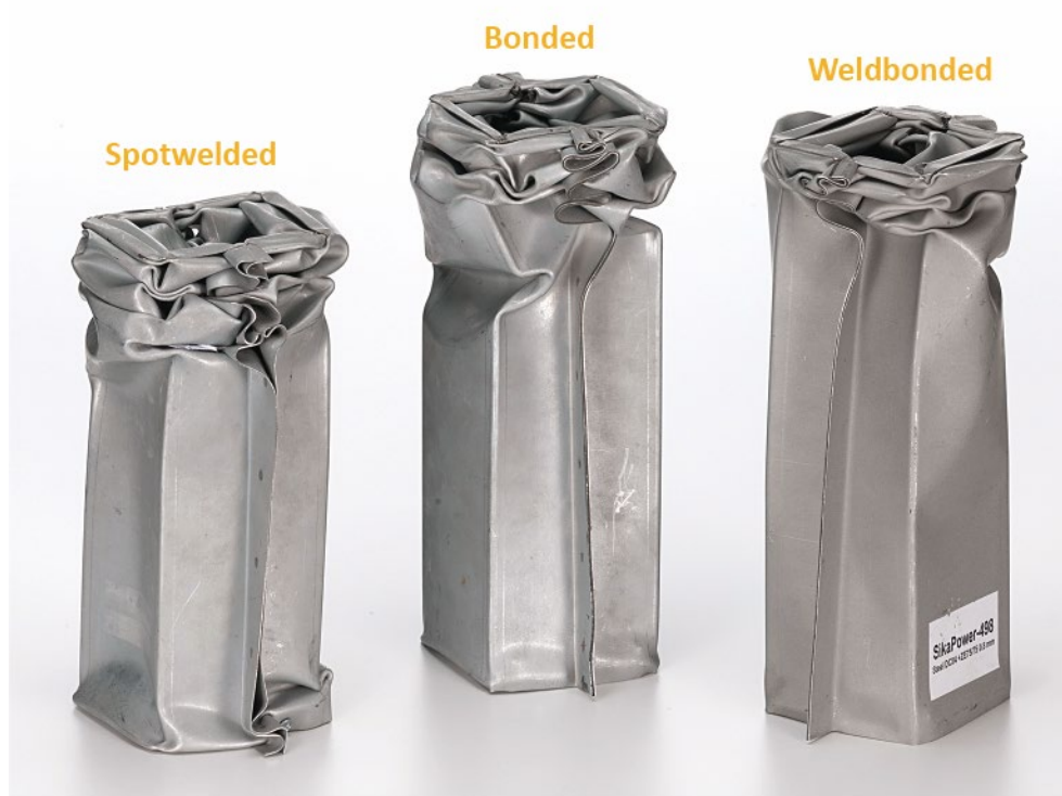
Figure 1: Spotwelded, bonded and weldbonded double hat profiles after crushing in a drop tower
