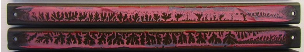
Figure 27: typical fracture surface showing viscous fingering
